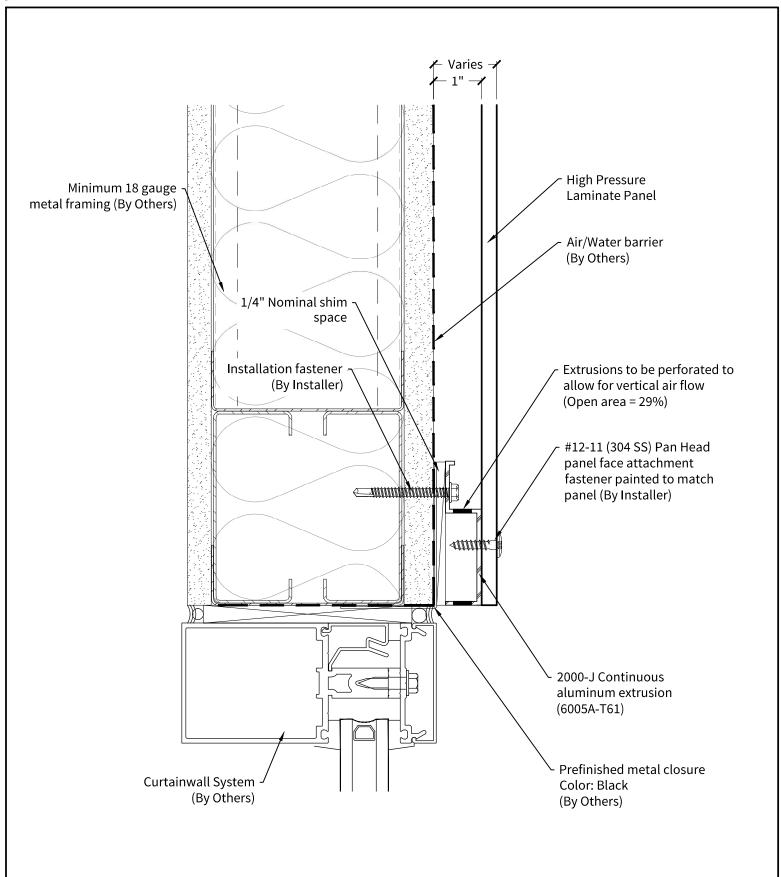
System 2000 **HPL Rainscreen** Detail: 8 Typical Window Head Detail
