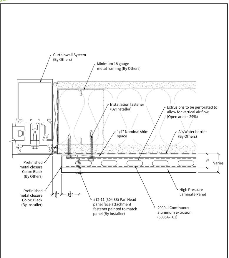
System 2000 **HPL Rainscreen** Detail: Typical Termination at Window Jamb
